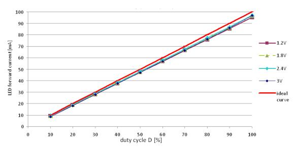
Figure 4. PWM Dimming Duty Cycle Versus LED Current
