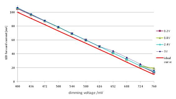
Figure 2. Analog Dimming Voltage Versus LED Current
