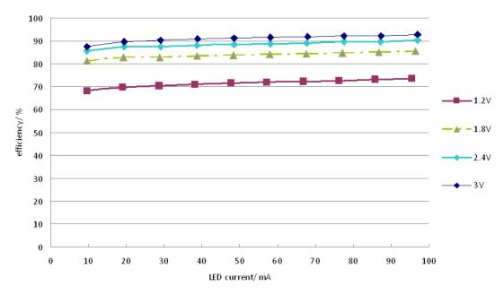
Figure 3. PWM Dimming Efficiency Versus LED Current
