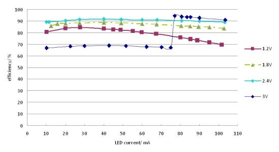
Figure 1. Analog Dimming Efficiency Versus LED Current
