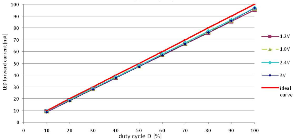
Figure 4. PWM Dimming Duty Cycle Versus LED Current
