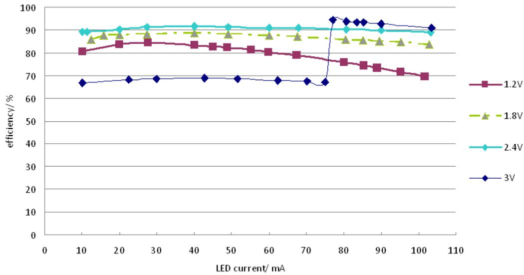
Figure 1. Analog Dimming Efficiency Versus LED Current
