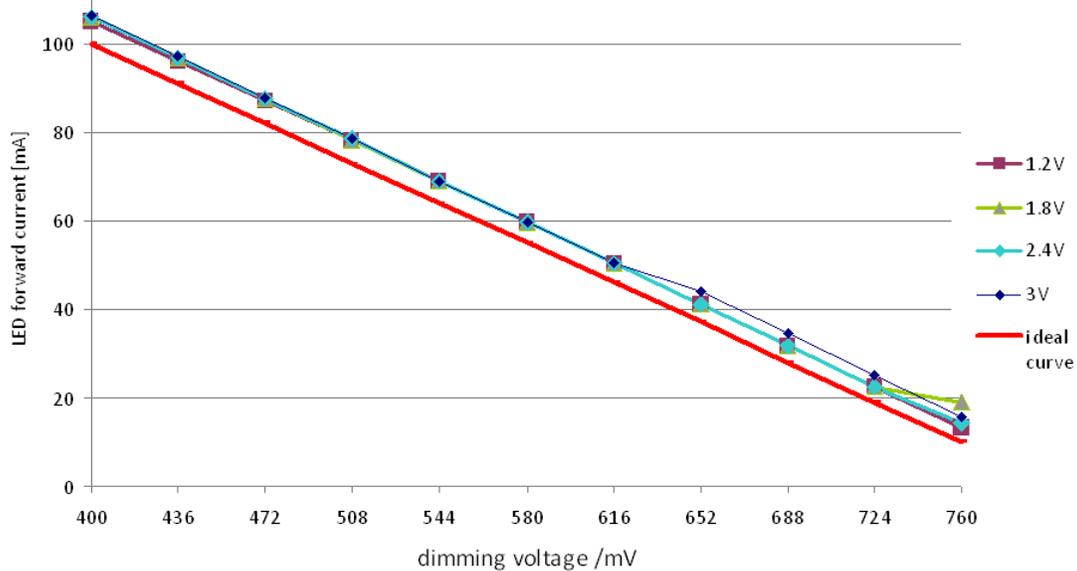
Figure 2. Analog Dimming Voltage Versus LED Current
