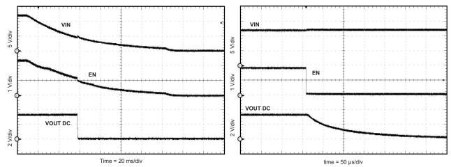
Figure 18. Shutdown Relative to VIN
