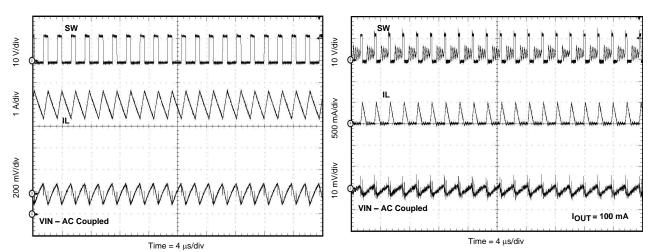
Figure 10. Input Voltage Ripple CCM
