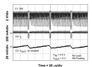
Figure 20. Low Dropout Operation
