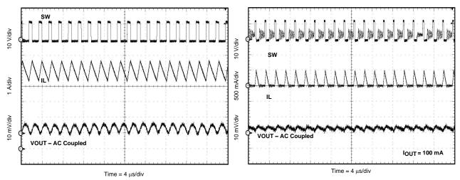
Figure 12. Output Voltage Ripple CCM
