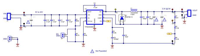
Figure 2. TPS54540EVM-558 Schematic
