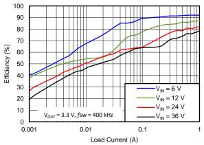
Figure 4. Light-Load Efficiency
