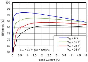
Figure 3. Efficiency Versus Load Current
