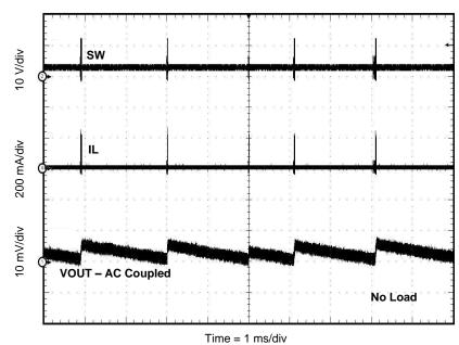
Figure 14. Output Voltage Ripple Eco-mode
