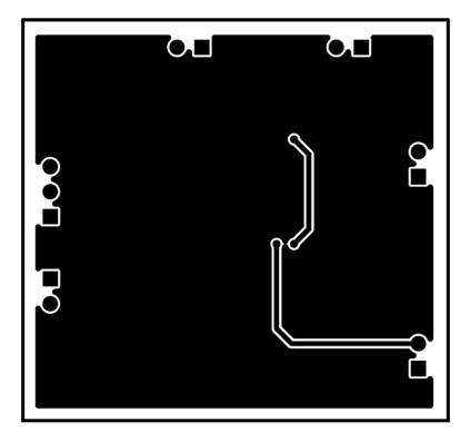
Figure 5. Bottom Layer Routing
