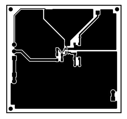
Figure 4. Top Layer Routing
