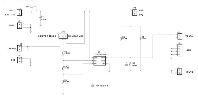
Figure 6. TPS3700EVM-202 Schematic
