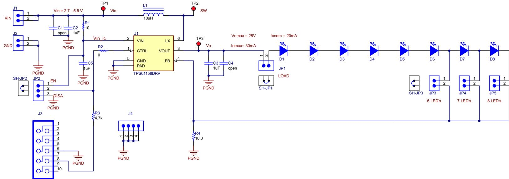
Figure 11. TPS61158EVM-565 Schematic
