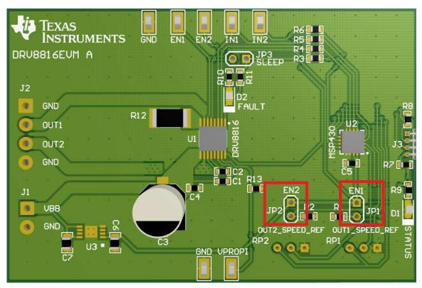
Figure 2. ENABLE Jumpers (EN1 and EN2)
