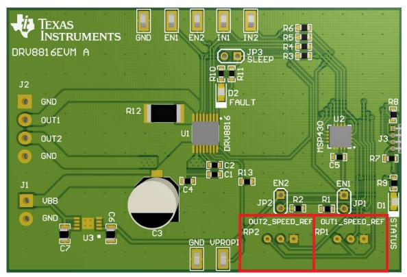
Figure 4. Speed Adjust Potentiometer (RP1 and RP2)
