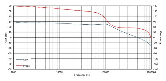
Figure 3. Loop Response for the TPS62684 (VIN = 5 V, Load = 1600 mA)
