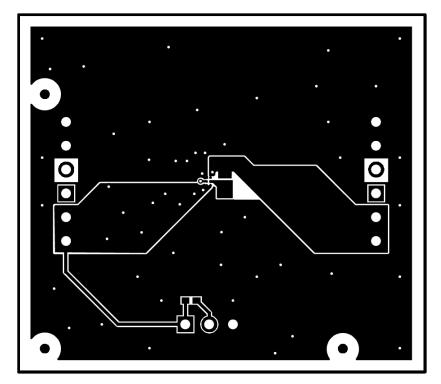
Figure 5. TPS62684EVM-647 Top Copper (Top View)
