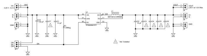
Figure 1. TPS62684EVM-647 Schematic
