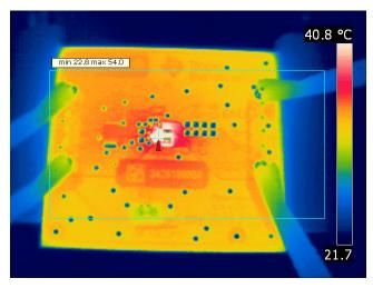
Figure 2. Thermal Performance for the TPS62684 (VIN = 5.5 V, Load = 1600 mA)
