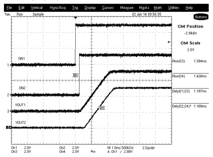
Figure 7. TPS22968EVM-007  $t_R$  with VIN=5V, CT=1nF and Load =10 $\Omega$ .
