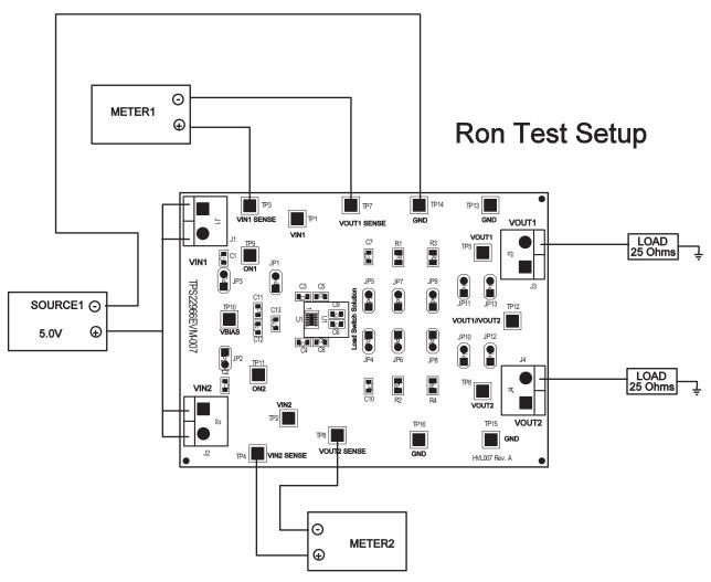
Figure 5. TPS22968EVM-007 Recommended Ron Test Set Up
