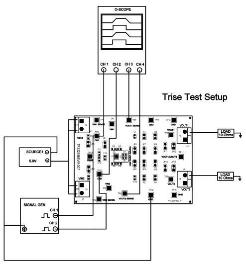
Figure 6. TPS22968EVM-007 Recommended Trise Test Set Up
