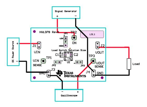
Figure 6. Slew Rate Setup
