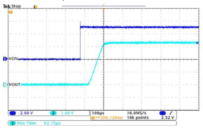
Figure 7. TPS22914/15 Vout  $t_R$  Example (V<sub>IN</sub> = 3.3V,  $R_L$  = 10 $\Omega$ )
