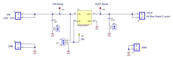
Figure 1. TPS22914/15EVM-078 Schematic
