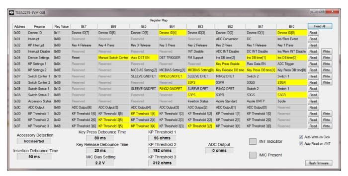
Figure 20. EVM GUI Settings When Using On-Board Keys
