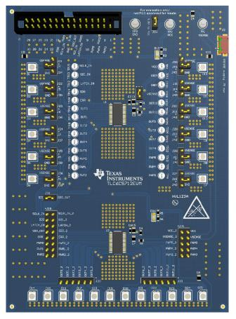
Figure 1. Top View of the TLC6C5712-Q1EVM PCB
