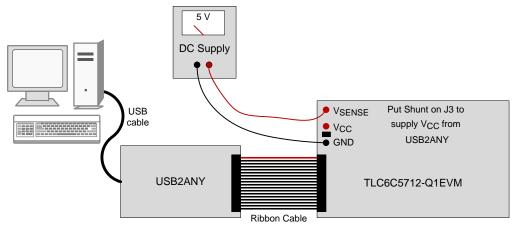
Figure 2. Hardware Setup for TLC6C5712-Q1EVM
