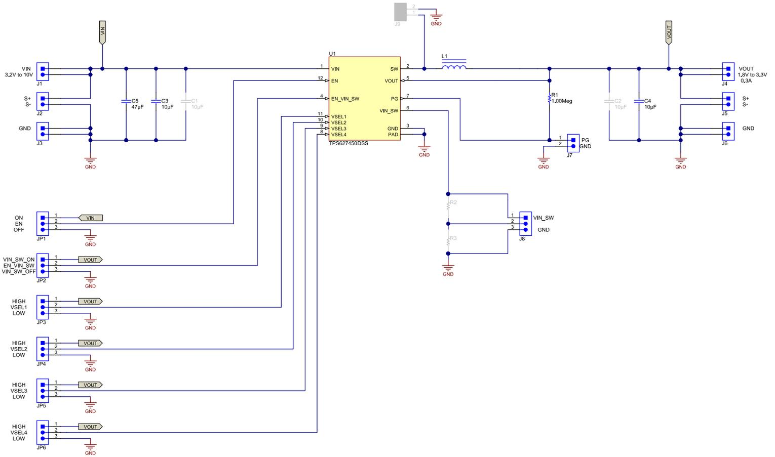
Figure 5-1. TPS62745EVM-622 Schematic
