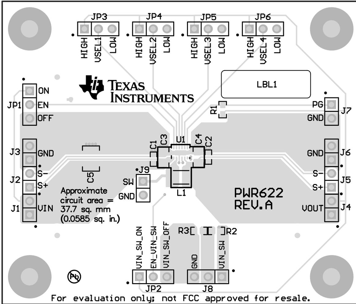
Figure 4-1. Assembly Layer
