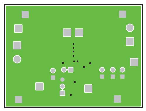
Figure 7. TPS22965NEVM PCB (Bottom)
