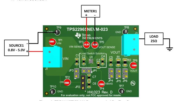
Figure 3. TPS22965EVM-023 Recommended R<sub>ON</sub> Test Setup
