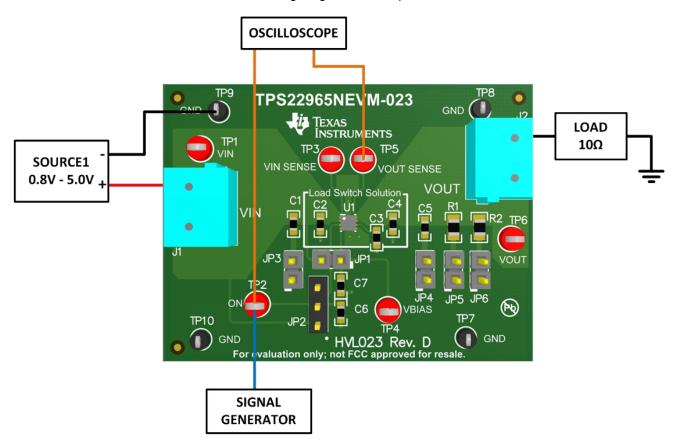
Figure 4. TPS22965NEVM Recommended AC Parameter Test Setup
