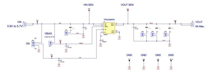
Figure 2. TPS22965NEVM Schematic
