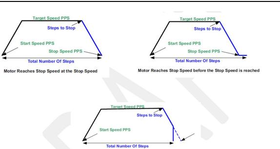
Motor runs out of Steps before reaching Stop Speed Figure 8. Three Stopping Conditions and Action Taken
