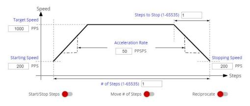
Figure 5. Motor Controls Enabled
