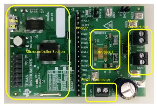
Figure 1. Typical Board Configuration (EVM Provided may Vary)
