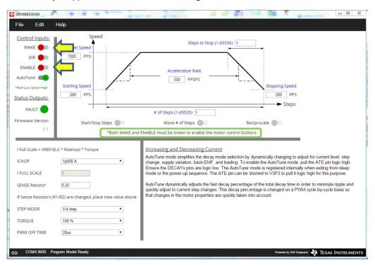
Figure 4. Wake and Enable Toggle Buttons
