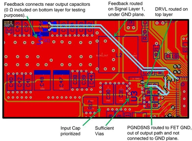
Figure 11. EVM Layout of Controllers
