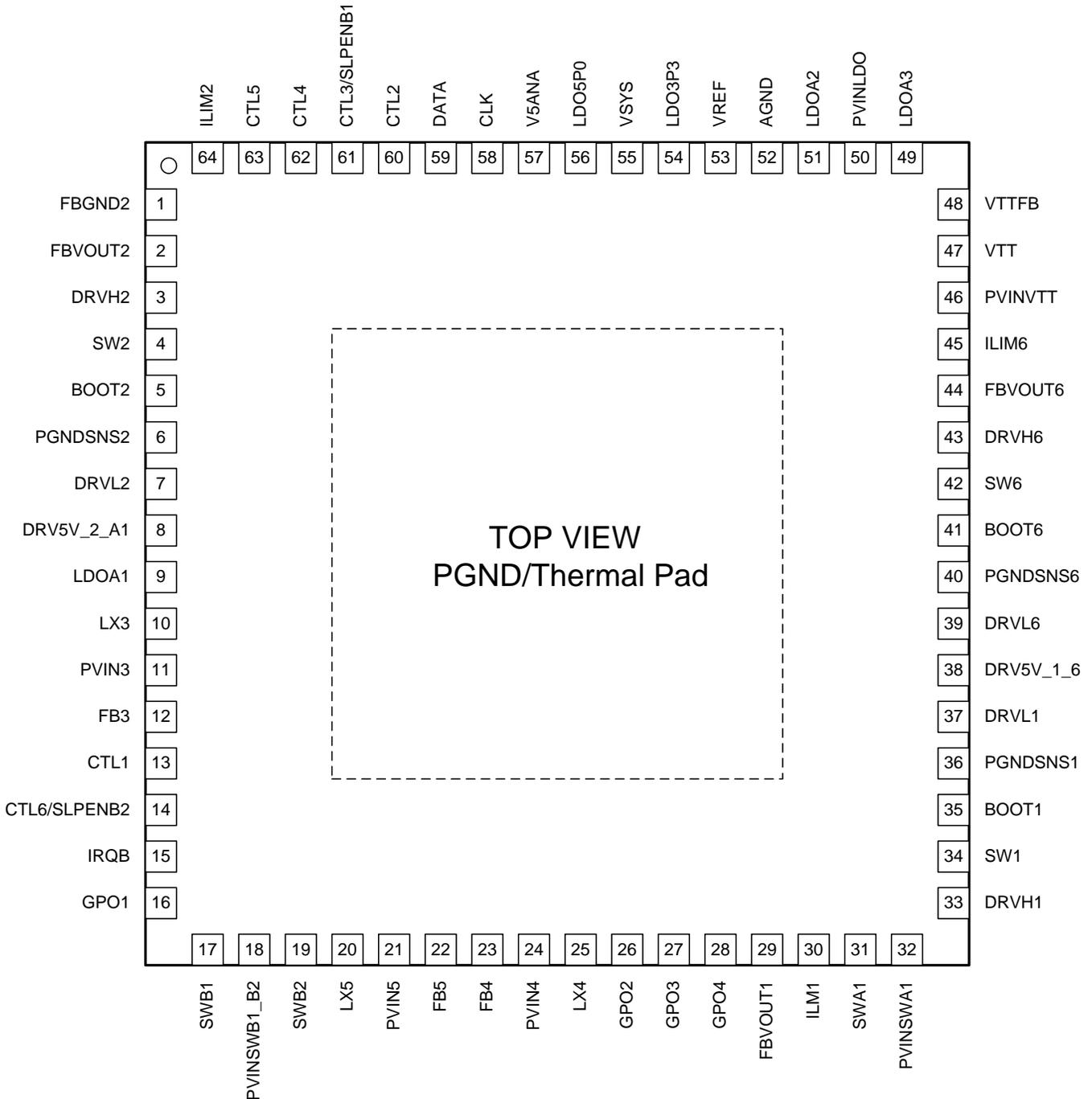
**Figure 5. Device Package and Pin Locations**
