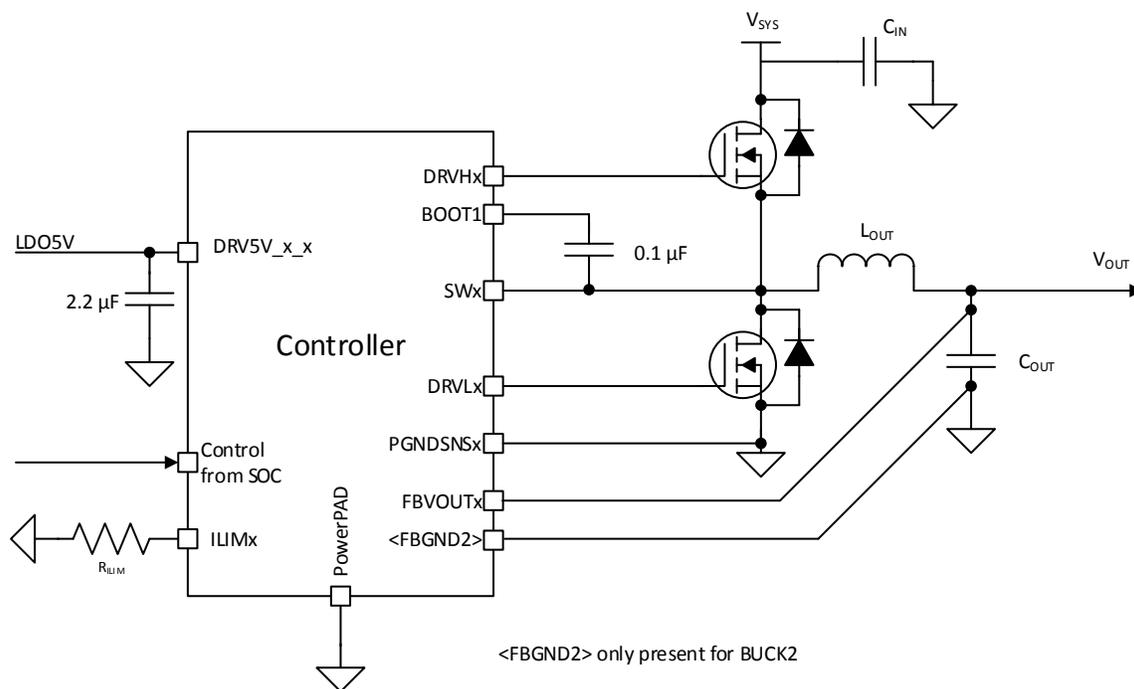
Figure 2. Controller Diagram
