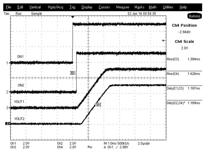
Figure 6. TPS22968NEVM  $t_R$  with VIN = 5 V, CT = 1 nF and Load = 10  $\Omega$ .
