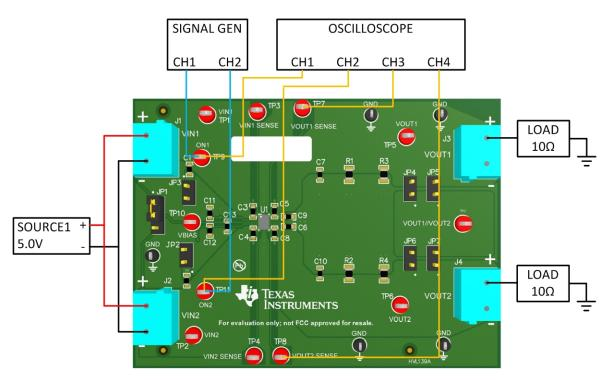
Figure 5. TPS22968NEVM Recommended t<sub>R</sub> Test Set Up
