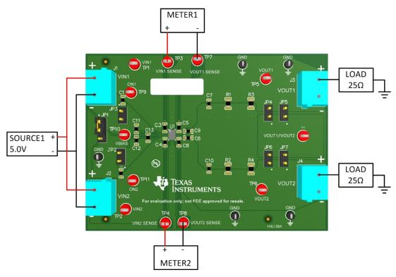
Figure 4. TPS22968NEVM Recommended  $R_{ON}$  Test Set Up
