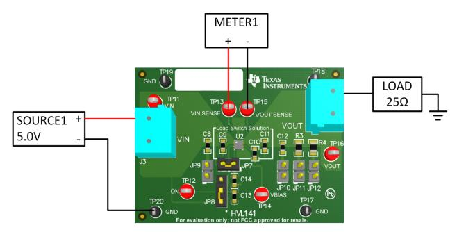
Figure 3. R<sub>on</sub> Test Setup
