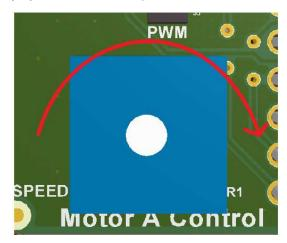
**Figure 3. Motor Speed Control Potentiometer**
