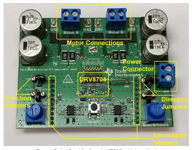
Figure 1. Typical Board Configuration (EVM Provided may Vary)
