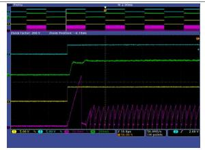
Ch1: DDRV voltage; Ch2: PWM input,
