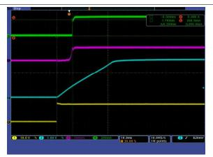
Ch1: Input voltage; Ch2: SS pin voltage;
