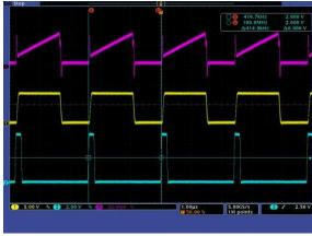
Ch1: GATE voltage; Ch2: SYNC input, TP2;
