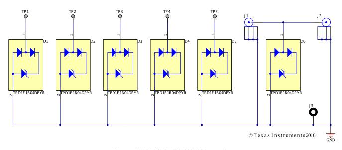
Figure 4. TPD1E1B04EVM Schematic
