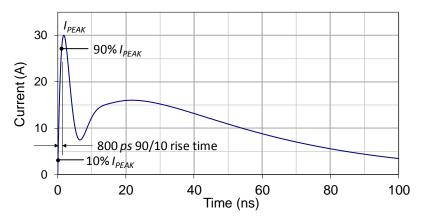
Figure 1. Ideal Contact Discharge Waveform of the Output Current of the ESD Simulator at 8-kV
