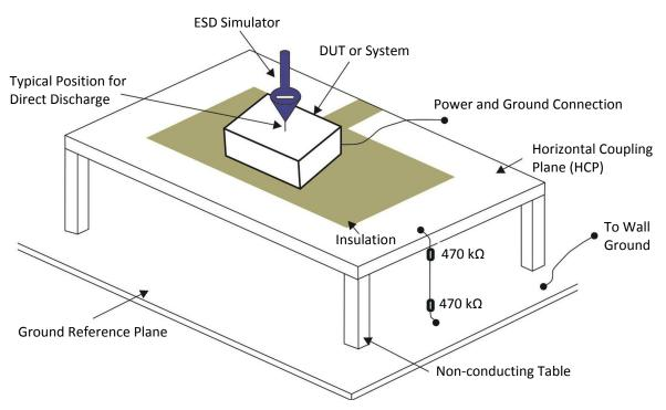
Figure 2. System Level ESD Test Setup
