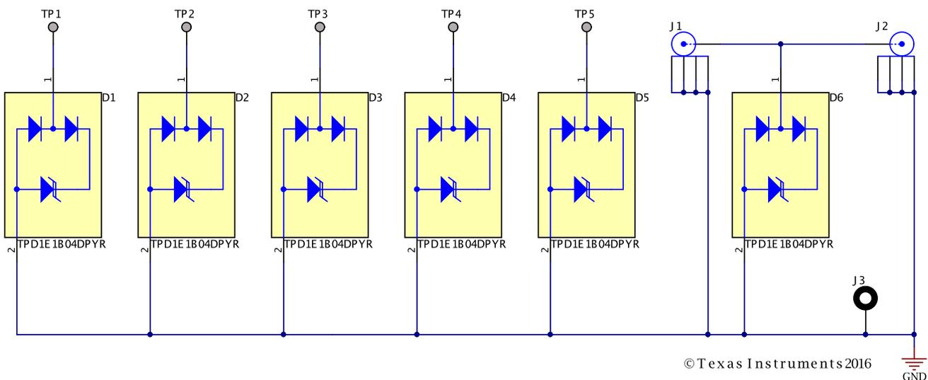
Figure 4. TPD1E1B04EVM Schematic
