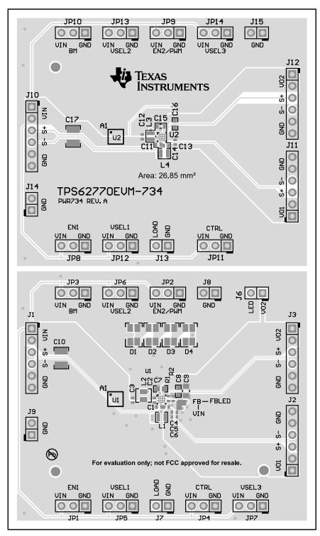
Figure 1. Assembly Layer
