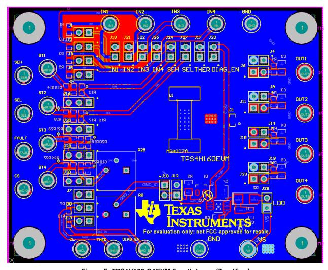
Figure 5. TPS4H160-Q1EVM Fourth Layer (Top View)
