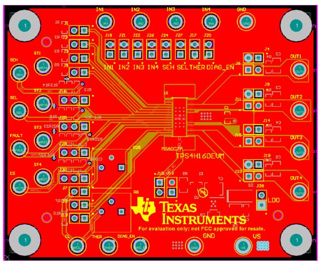
Figure 2. TPS4H160-Q1EVM First Layer (Top View)
