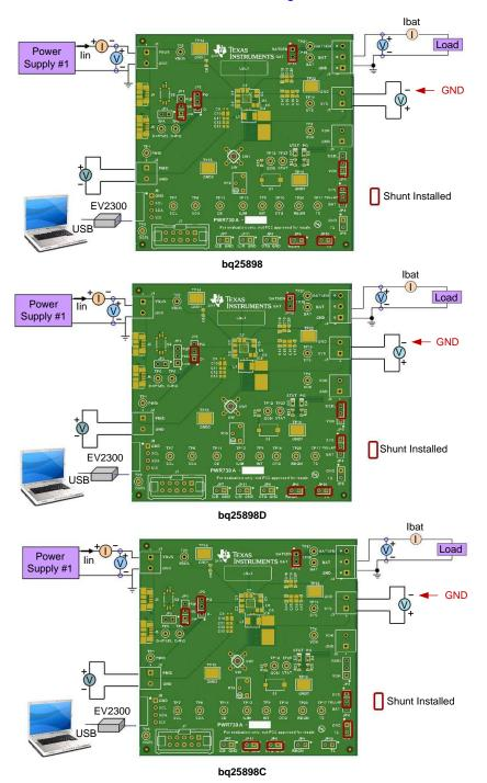
Figure 2. Original Test Setup for bq25898X
