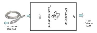
Figure 1. Connections of the EV2300 Kit
