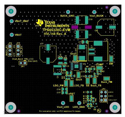
Figure 5. Top Assembly Layer
