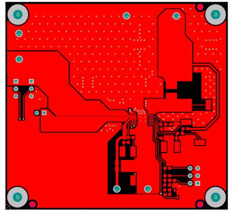
Figure 6. Top Layer Routing
