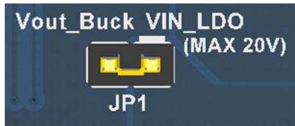
Figure 4. VIN\_LDO Jumper
