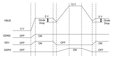
Figure 2. Switching Between 5 V and 12 V Using GDNG, G5V, and GDPG
