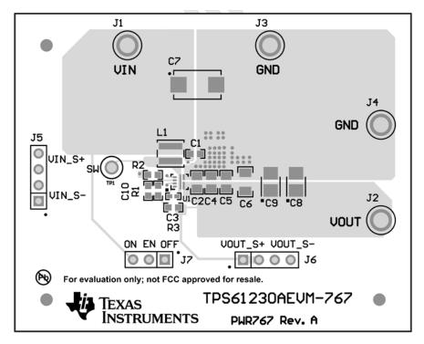
Figure 2. Top Side of the TPS61230A Evaluation Module
