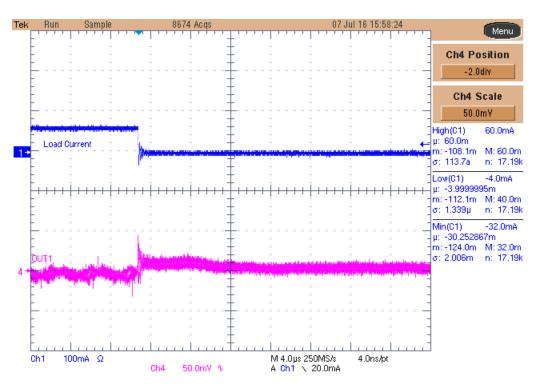
Figure 17. PFM Load Transient Response: VOUT1 Falling Edge
