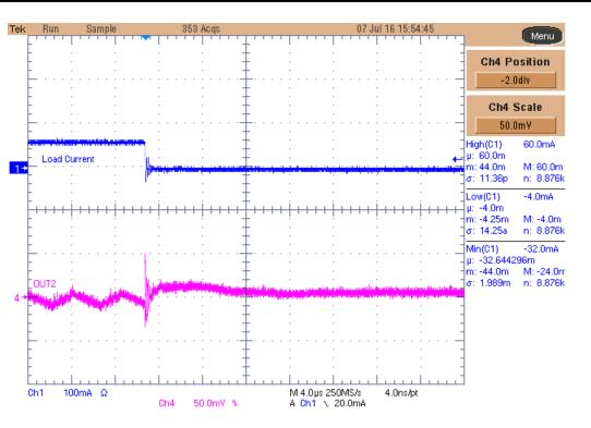
Figure 19. PFM Load Transient Response: VOUT2 Falling Edge
