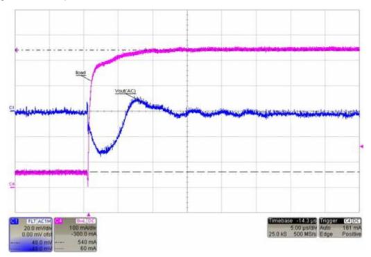
Figure 12. PWM Load Transient Response: VOUT1 Rising Edge
