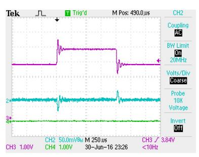
Figure 21. Line Transient Response: VOUT2
