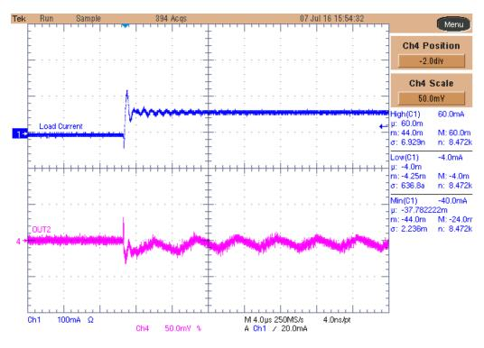
Figure 18. PFM Load Transient Response: VOUT2 Rising Edge
