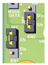
Figure 9. Enable Jumper Settings
