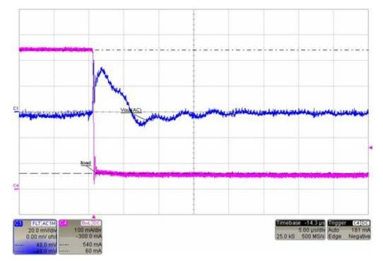
Figure 13. PWM Load Transient Response: VOUT1 Falling Edge
