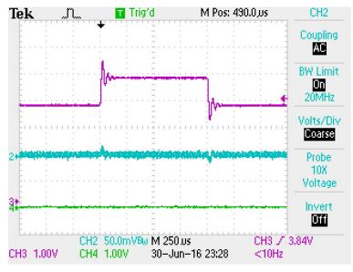
Figure 20. Line Transient Response: VOUT1
