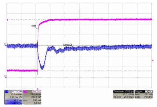
Figure 14. PWM Load Transient Response: VOUT2 Rising Edge
