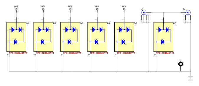
Figure 4. TPD1E0B04DPYEVM Schematic
