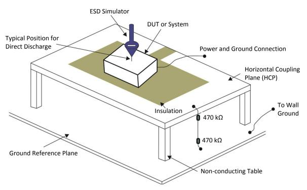
Figure 2. System Level ESD Test Setup
