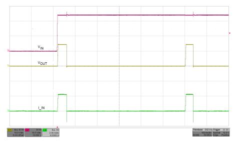
Figure 4. J5/J12 = 2-3 Position, Current Limit (2.23 A), Auto-Retry Mode
