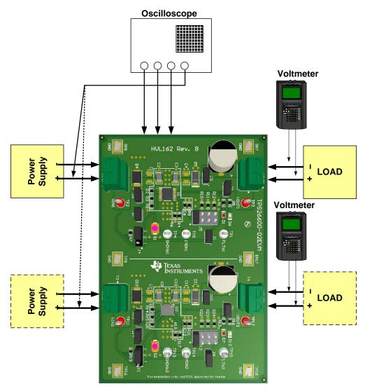
Figure 2. EVM Test Setup
