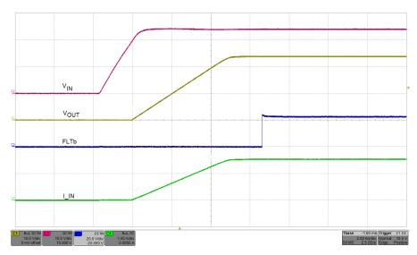
Figure 3. Output Voltage Start-Up Waveform
