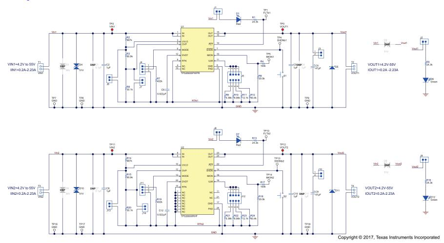
Figure 1. TPS26600-02EVM Schematic
