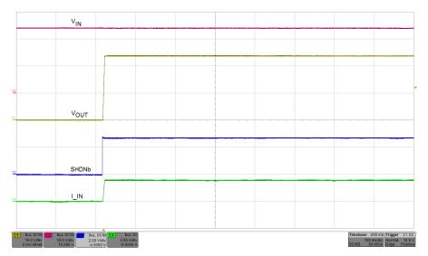
Figure 6. Restart From Latch-Off Mode
