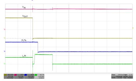
Figure 8. Output Short-Circuit Protection
