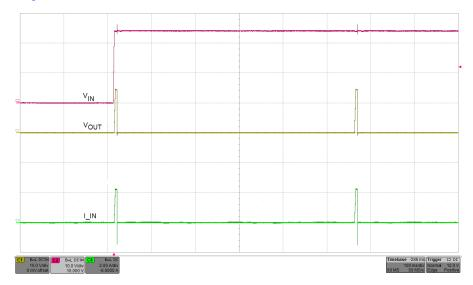
Figure 7. J5/J12 = Floating, Current Limit (2.23 A), Circuit Breaker With Auto-Retry Mode
