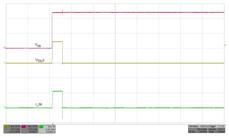
Figure 5. J5/J12 = 1-2 Position, Current Limit (2.23 A), Latch-Off Mode
