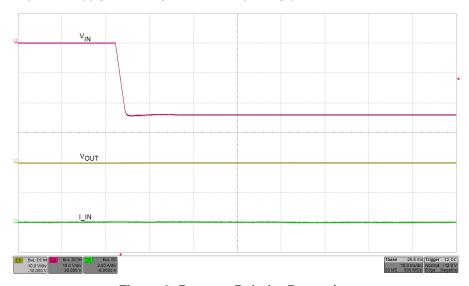
Figure 9. Reverse Polarity Protection
