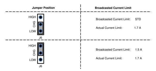
Figure 7. Jumper J6 Setting for Each Broadcasted Current Level
