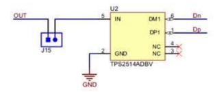
Figure 11. Schematic of TPS2514A Device Section
