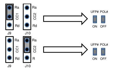
Figure 10. Connecting a Full-Featured USB Type-C<sup>™</sup> Cable to TPS25820/21EVM
