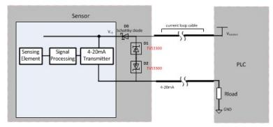
Figure 2. 2-Wire Protection Model
