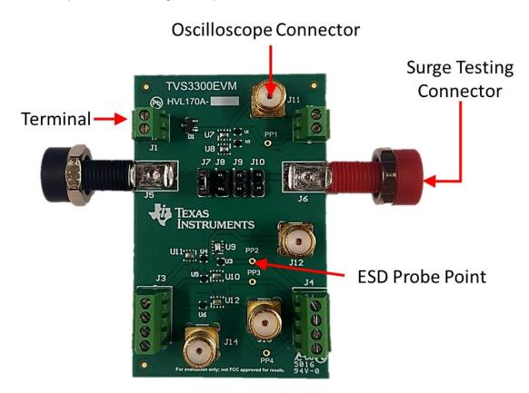
Figure 1. TVS3300DRV EVM Circuit Board Setup
