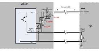
Figure 4. 3-Wire Digital I/O Protection Test Circuit
