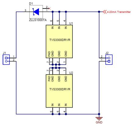
Figure 3. 2-Wire Protection Test Circuit
