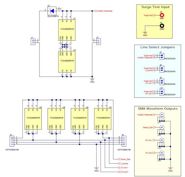
Figure 7. TVS3300DRV EVM Board Schematic
