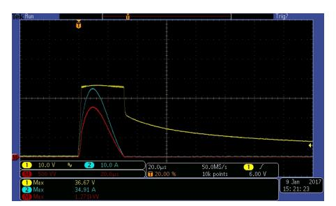
Figure 6. TVS3300DRV Surge Test Waveform
