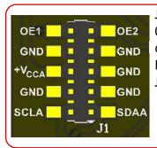
J1 is the connector designed to be mated with any  $I^2C$  master via 0.100" headers. J1 allows for power connection (+ $V_{CCA}$ ), ground connection, OE1 for U1, OE2 for U2, SDA, and SCL data lines. U2 is by default loaded with TCA9802. Connect + $V_{CCA}$  to the EVM using J1-6.
