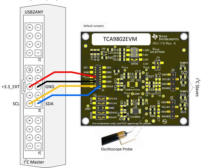
Figure 4. Example: USB2ANY I<sup>2</sup>C Master Connected to the TCA9802EVM
