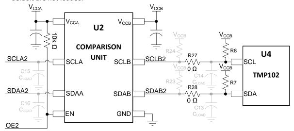
The EVM has also been setup to be able to directly probe onto the SCLB2 and SDAB2. There are large vias that facilitate the scope probe tips and probe ground connections. This was designed to minimize the ground loop to minimize noise being picked up by the probe. This allows for capturing clean waveforms. NOTE: If evaluating a device such as the TCA9517 at U2, calculate the appropriate pullup resistor and load them on to the desired pullup resistor location on the B side of the device.
