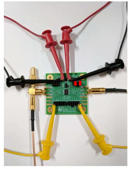
Figure 8. Typical LSF-EVM Setup
