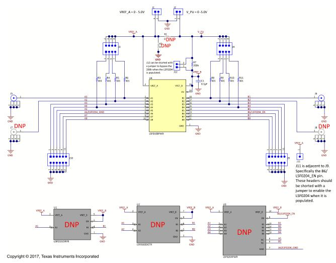
Figure 13. LSF-EVM Schematic (Zoom for Higher Resolution)
