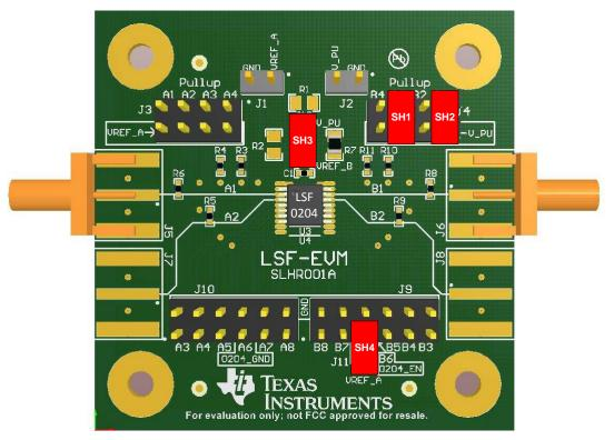
Figure 9. LSF0204 Board Setup
