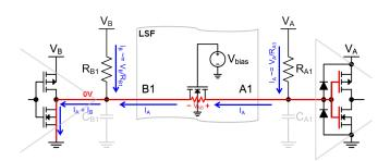
Figure 7. LSF Pass Transistor LOW-State Operation
