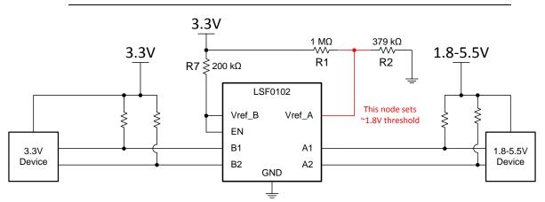
Figure 10. LSF0102 Single-Supply Operation Setup
