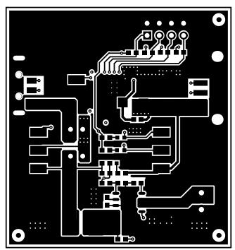
Figure 4. Top Side Routing
