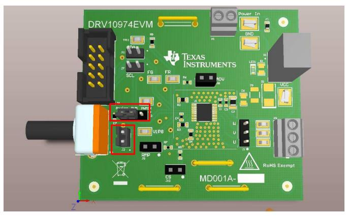
Figure 3. Jumper Configurations for Controlling Speed With Analog Voltage
