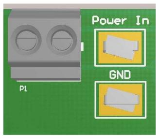
Figure 5. Power Input Terminal Block (P1)
