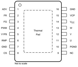
Figure 7. DRV10974PWP Pinout
