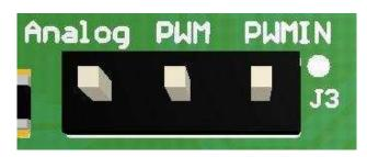
Figure 11. Speed Command Input Select Header (J3)
