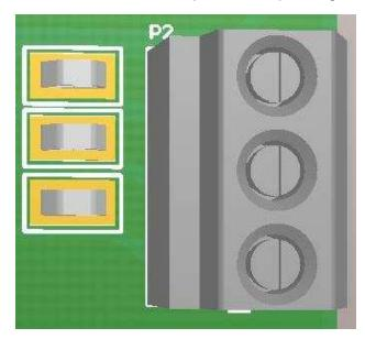
Figure 6. Motor Phase Windings Input Terminal Block (P2)
