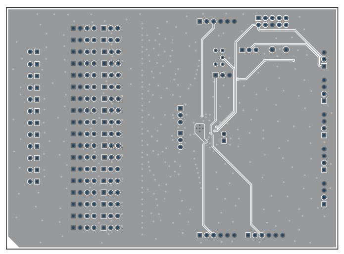
Figure 6. TPS65680 EVM Bottom Layer (Bottom View)
