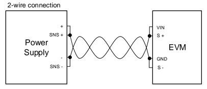
Figure 2. Two- and Four-Terminal Connection
