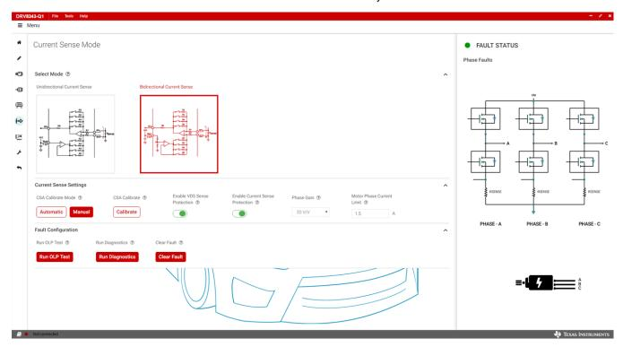
Figure 11. DRV8343x-Q1EVM GUI - Current Sense Mode Page
