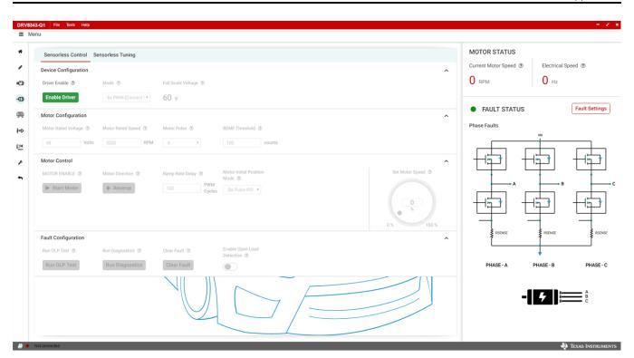
Figure 9. DRV8343x-Q1EVM GUI - Sensorless Page (Motor Control and Tuning)
