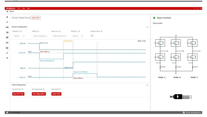
Figure 12. DRV8343x-Q1EVM GUI - Smart Gate Drive Page
