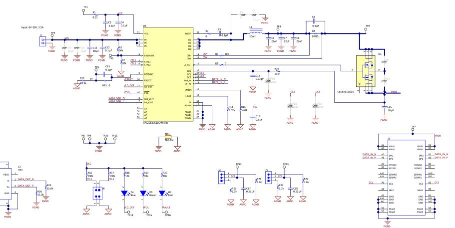
Figure 1. TPS25830Q1EVM-040 Schematic
