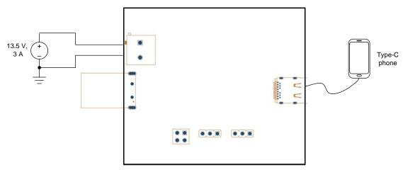
Figure 2. EVM Setup for Charging USB Type-C<sup>™</sup> Device
