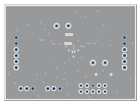
Figure 4. TPS6381xEVM PCB - Signal Layer 1 (Top View)
