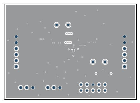
Figure 5. TPS6381xEVM PCB - Signal Layer 2 (Top View)
