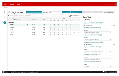
Figure 11. GUI Register Map Screen
