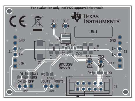
Figure 2. TPS6381xEVM PCB - Assembly Layer
