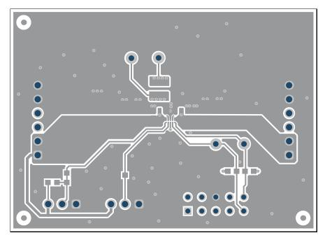
Figure 3. TPS6381xEVM PCB - Top Layer
