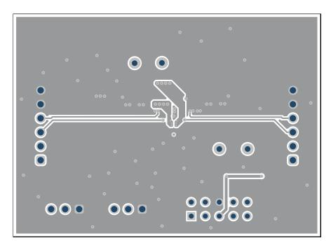
Figure 6. TPS6381xEVM PCB - Bottom Layer (Top View)
