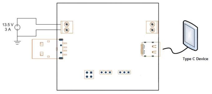
Figure 2. EVM Setup for Charging USB Type-C™ Device
