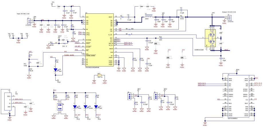
Figure 9. TPS25831Q1EVM-062 Schematic
