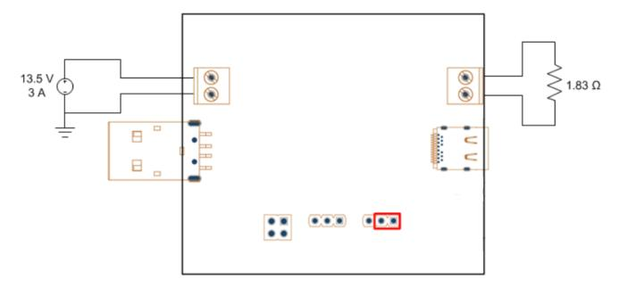
Figure 1. EVM Setup For Testing Buck Converter
