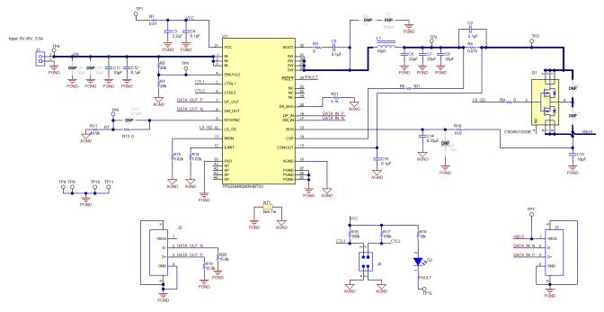
Figure 8. TPS25840Q1EVM-079 Schematic
