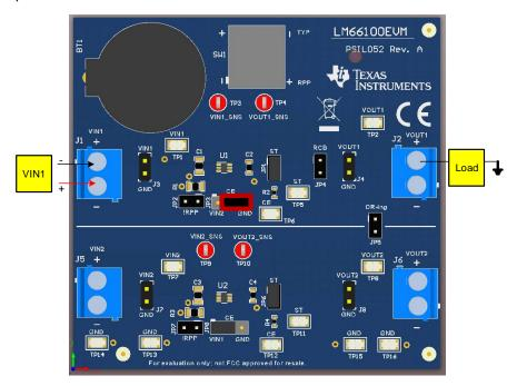
Figure 7. Reverse Polarity Protection Test Setup
