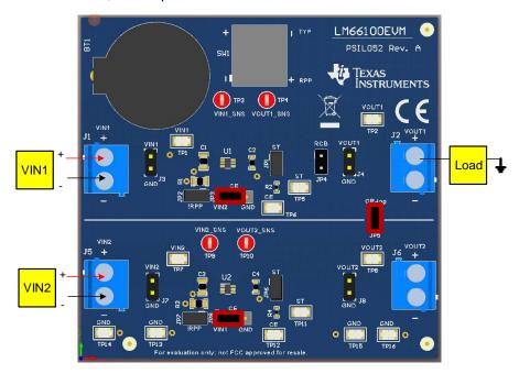
Figure 5. ORing Test Setup
