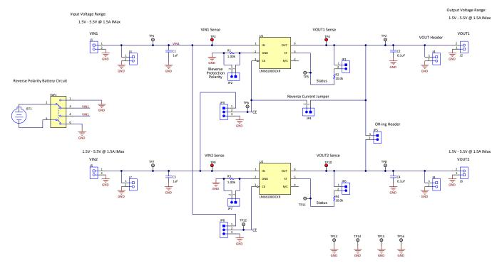
Figure 1. LM66100EVM Schematic
