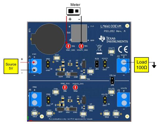
Figure 4. Ron Test Setup
