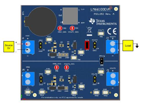
Figure 6. Reverse Current Blocking Test Setup
