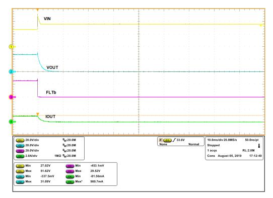
Figure 6. LM76202-Q1EVM Output Overvoltage Protection (VIN = 36 V, ILIM = 2.23 A, ROUT = 28  $\Omega$ , MODE = RTN)
