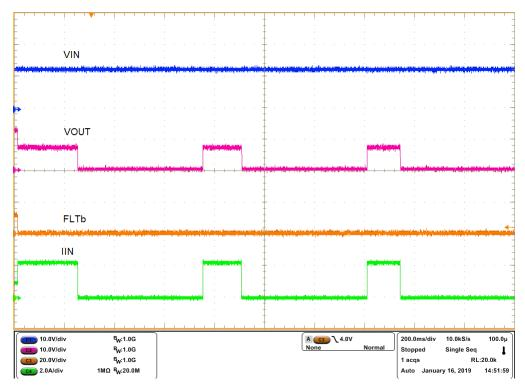
Figure 4. LM76202-Q1EVM Current Limit Operation (VIN = 12.5 V, ILIM = 2.23 A, ROUT = 3  $\Omega$ , MODE = RTN)
