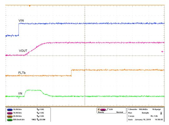
Figure 3. LM76202-Q1EVM Output Slew Rate with Inrush Current Limiting (VIN = 12.5 V, CdVdT = 12 nF, COUT = 47  $\mu$ F, No-load)
