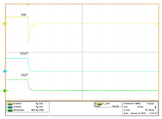
Figure 8. LM76202-Q1EVM Negative Input Voltage Transient Test (12-V battery voltage, transient voltage = -150 V,  $R_{\text{LOAD}} = 12 \Omega$ )
