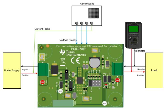
Figure 2. LM76202-Q1 EVM Setup
