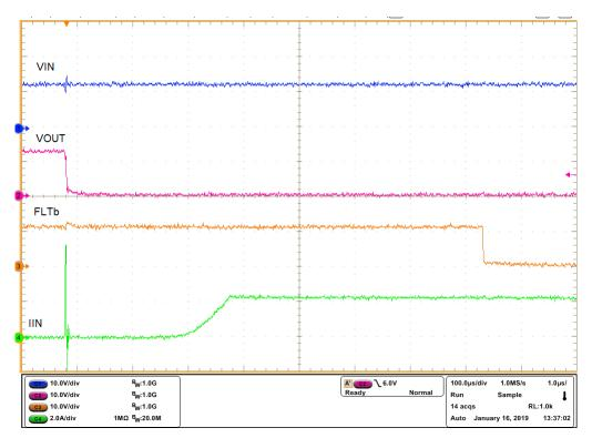
Figure 5. LM76202-Q1EVM Output Hot Short (VIN = 12.5 V, ILIM = 2.23 A, MODE = RTN)
