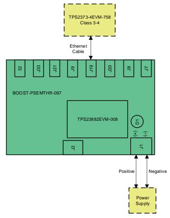
Figure 1. Basic Setup Using Autonomous Mode
