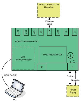
Figure 3. Advanced Setup Using LaunchPad™
