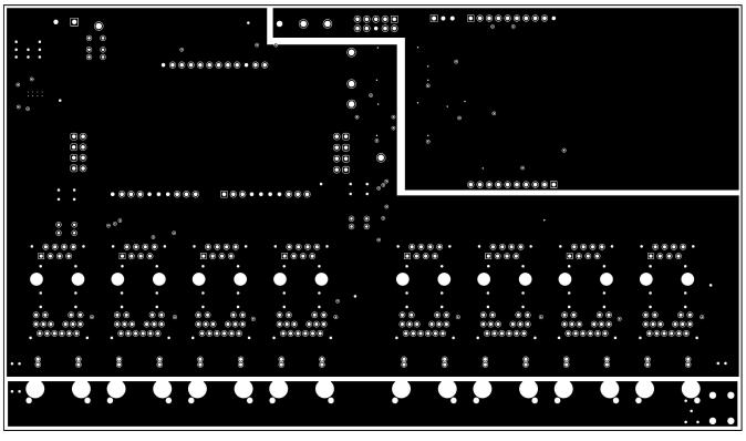
Figure 18. BOOST-PSEMTHR8-097 (Motherboard) Layer 2 Routing
