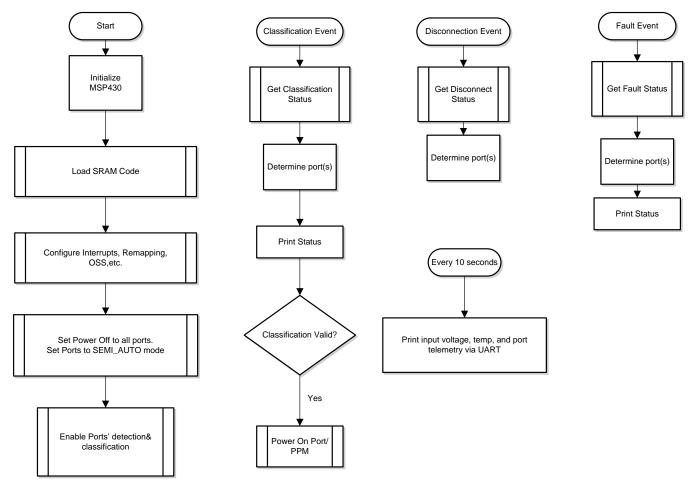
Figure 12. Semi Auto Mode System Software Structure
