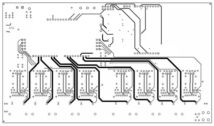
Figure 20. BOOST-PSEMTHR8-097 (Motherboard) Bottom Side Routing
