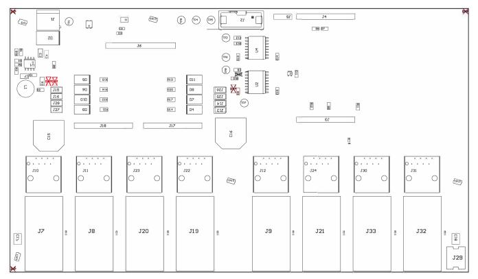
Figure 16. BOOST-PSEMTHR8-097 (Motherboard) Top Side Assembly
