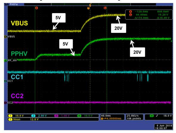
Figure 8. PD Transactions and VBUS Timing Waveform
