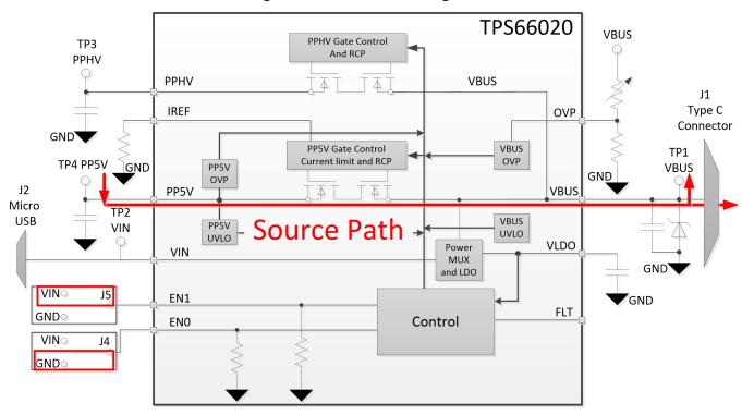
Figure 4. Source Path Configuration
