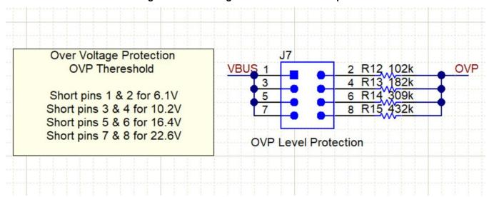
Figure 6. Overvoltage Protection Level Jumper
