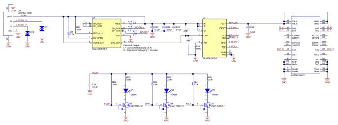
Figure 7. Type-A to USB Type-C<sup>™</sup> Converter
