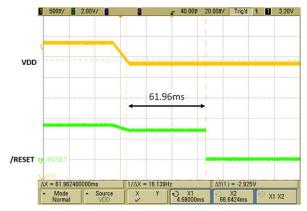
Figure 4-1. Sense Delay Oscilloscope Capture
