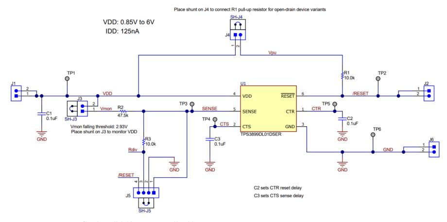
Place shunt on J5 pin 4-3 to create programmable push-button
