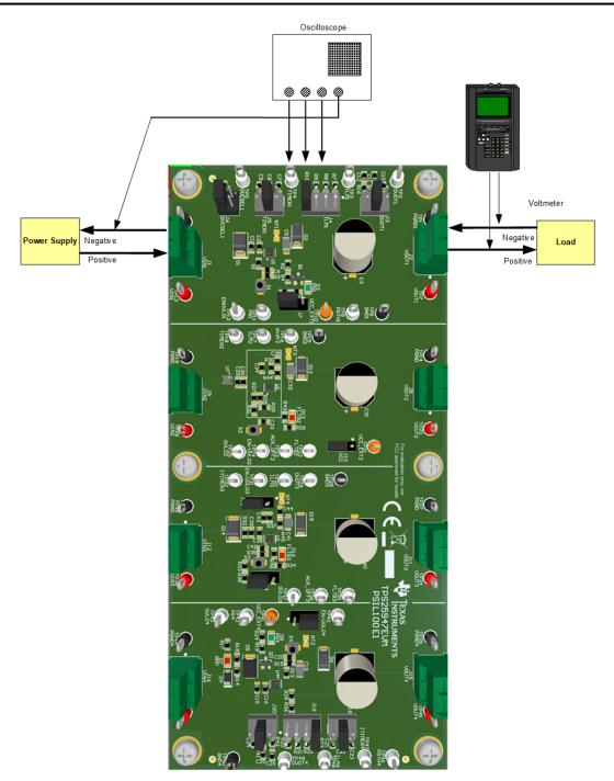
Figure 5-1. TPS25947EVM Setup with Test Equipment
