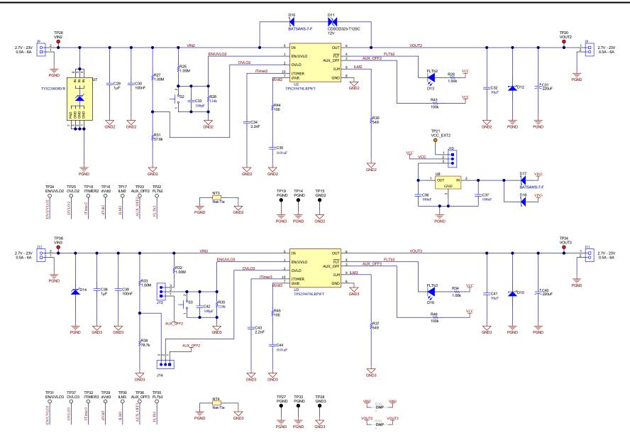
Figure 3-1. TPS25947EVM eFuse Evaluation Board Schematic
