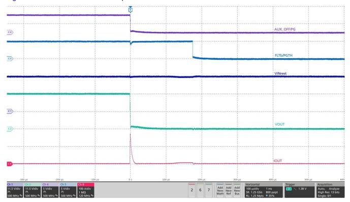
Figure 5-4. Output Hot-short response of TPS25947xx device at Vin = 23V, Cout = 10uF, ITIMER = OPEN, ILIM =  $549\Omega$
