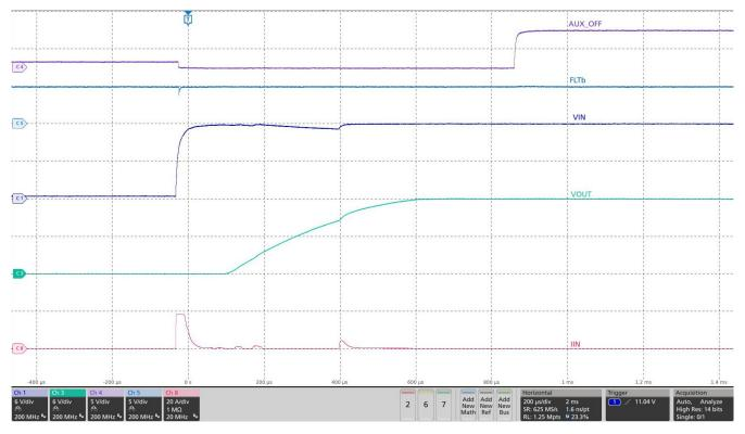
Figure 5-2. TPS259470x Output Rise Profile (VIN = 12 V, Cout=10uF, CdVdT = OPEN, ILIM =549Ω, No-load)
