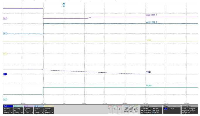
Figure 5-7. Priority PowerMux test on TPS259470x
