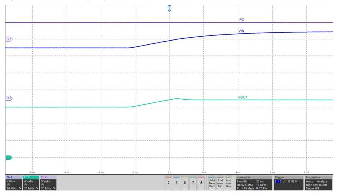
Figure 5-6. Over Voltage Protection Response of TPS259472x Device
