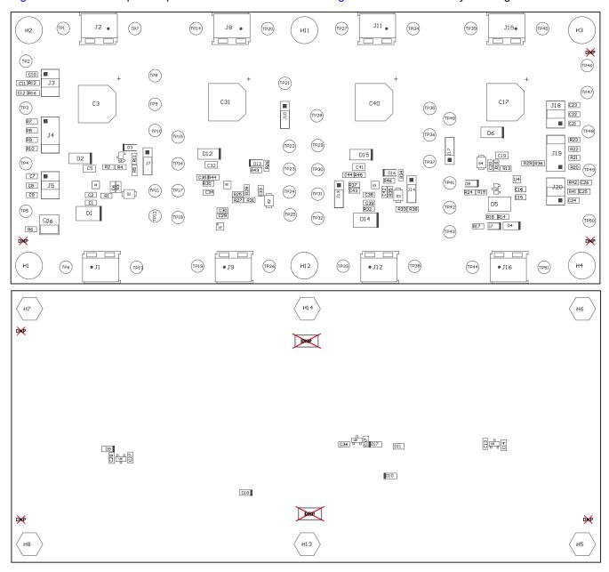
Figure 6-1. TPS25947EVM Board (a) Top Assembly (b) Bottom Assembly
