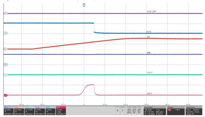
Figure 5-5. Test Waveform of Wakeup Into Output Short for TPS25947xx Device at Vin = 23V, dVdt = OPEN, Cout = 470 uF, ILIM =  $549\Omega$
